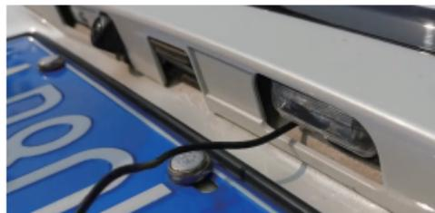
4. Connect the rear camera's power cable to the extension cable. After snaking your rear camera's extension cable, connect the power cable to your rear camera's extension cord.
