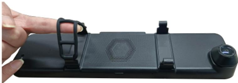
Step 2: Extend the straps around the back of the rear-view mirror and attach them to the bottom retaining hooks.
